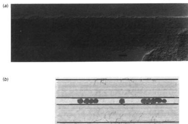
Fig. 2 (a) Micrograph of a cytochrome c_3 molecule (3.1 nm) and aggregates inside a nanotube. The protein can also be seen on the outside surface of the nanotubes. The scale bar is 5 nm. (b) Sketch of details in (a).
